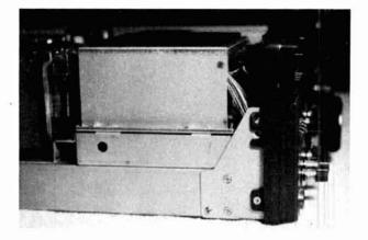
fig. 1. Front panel mounting bracket screws.
